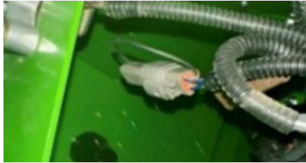
fig. 2C – CANDapter shown connected to the VANQUISH's CANbus port and USB on stand up models. VANQUISH's port is located under the tower below the display. FURY's port is located inside the controller compartment above the LH Drive Controller.
