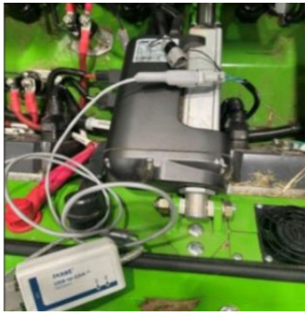
fig. 2A – CANDapter shown connected to the RIVAL's CANbus port and USB near the RH Drive Controller under the seat.
